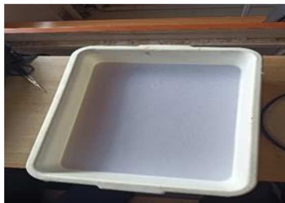
Figure 5: This is pulp solution of NaOH and H 2 O 2 in which deinking process done.
